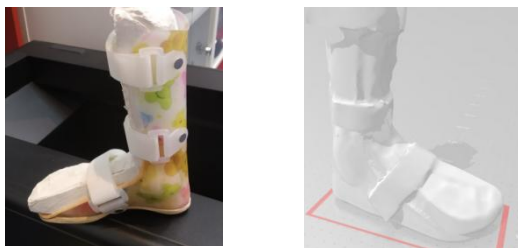
Fig. 2 Plaster copy of foot with orthoses as the base for shoe last design.
