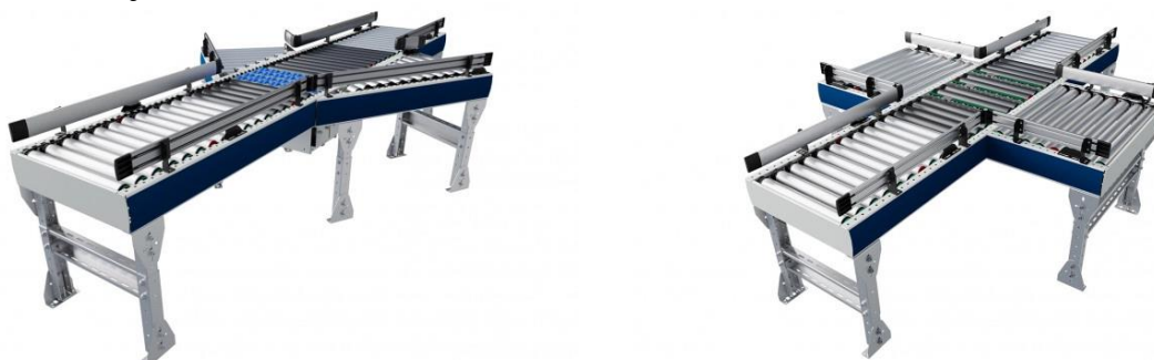
Fig. 7. Examples of roller conveyors usage for production objects overloading
