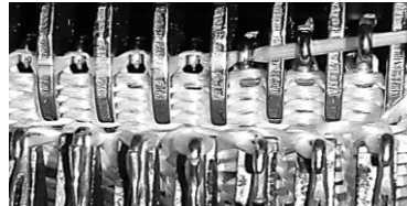
Fig. 2. The process of forming loops on a flat-knitting glove machine (PA-8-33)
