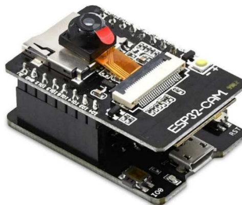
Fig. 2. External view of ESP32-CAM module with camera and USB interface board
