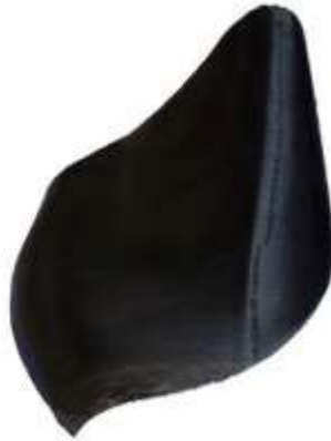
Fig. 1. Individual last cover made by 3D printing
