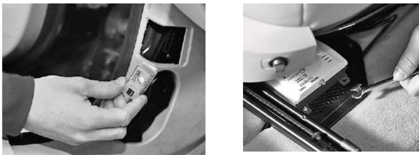
Fig. 1. TEXA Remote Diagnostic Block Transmitter
