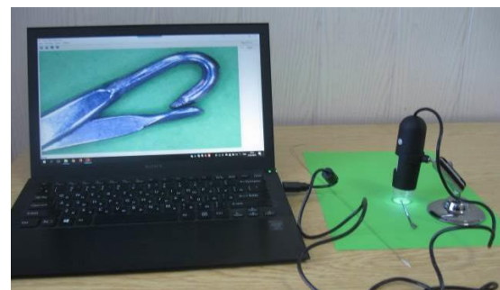
Figure 6 Setup for determining geometric dimensions of the structural elements I – IV of the threading system of the loom
